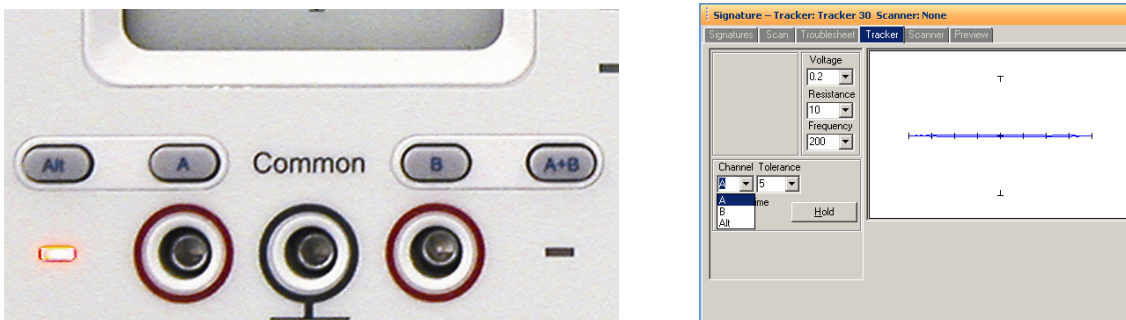
Figure 1-7 Channel A and Channel B shown on a Huntron ProTrack and in Workstation software
